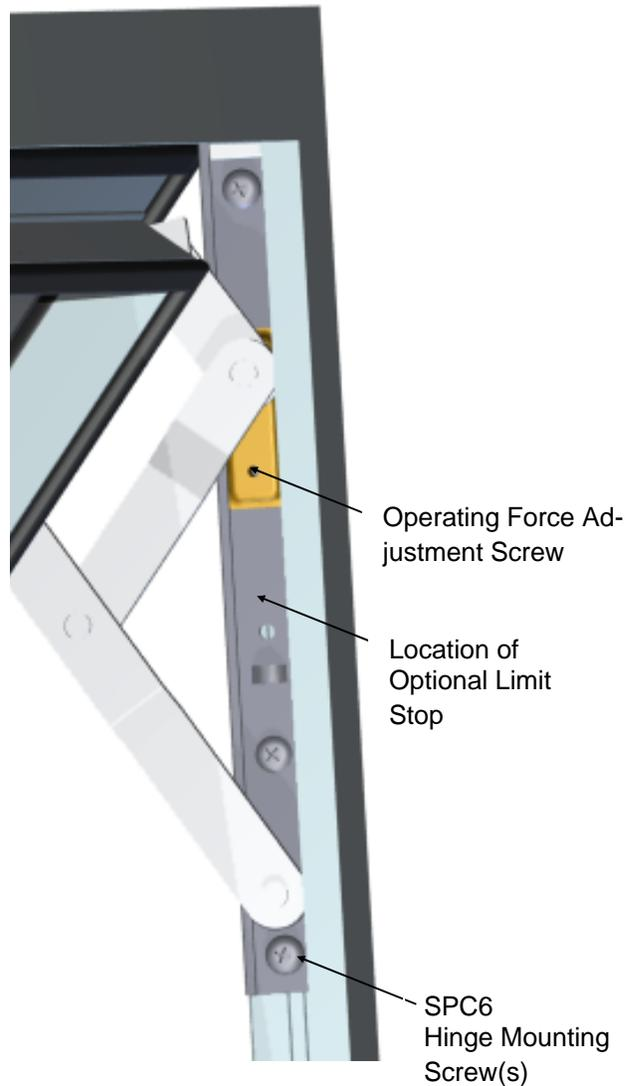
The hold open force for the vent can be adjusted by a set screw located in the hinge friction shoe. See Figure 25. Open the vent far enough to access the set screw. Turn the screw clockwise to increase the friction, counterclockwise will decrease the friction. Adjust both hinges equally, make small adjustments, and check operation.
